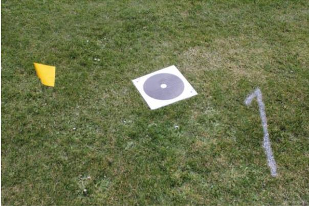
Figure 1: Ground control station and check point targets
