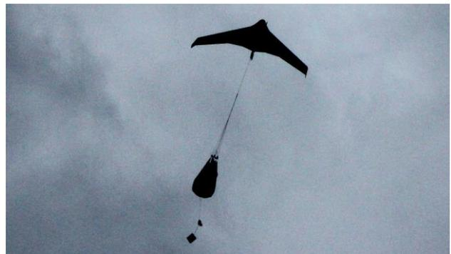
Figure 4: The C-Astral Bramor UAV during the initial deployment of its landing parachute.
