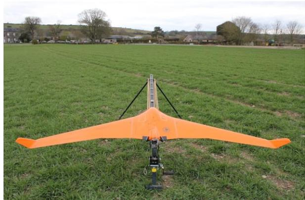
Figure 3: The C-Astral Bramor UAV on the catapult ready for launch.
