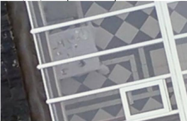
Figure 6: The detail of 1cm orthophotography can be seen here. This is a view looking down through the atrium over the dinning area of the surveyed hotel. Note the cutlery on the table.
